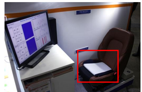
Cushion with built-in SR sensor installed in seat
