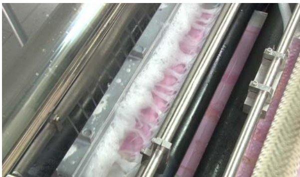
Finishing the plate with the brush while applying water
