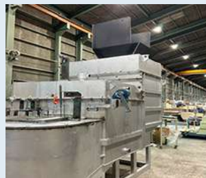
Reduction of radiant heat from equipment using heat-shielding coating on molds
