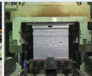
Reduction of radiant heat from equipment using heat-shielding coating on molds
