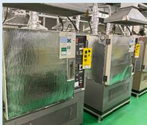
Drying oven insulated with in-house developed insulation material (Finesulight®)
