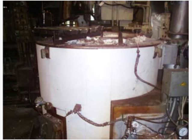
Aluminum melting furnace before installation (left)/ Finesulight is applied around aluminum melting furnace (right)
