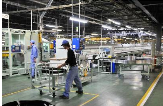
60 m-long high-pressure hose manufacturing line
